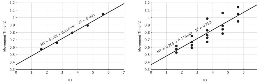
(a) A regression analysis using average MT results for every  $ID$  value. A very good fit of data to model is due to the averaging of data points, concealing the underlying nature of the data.
