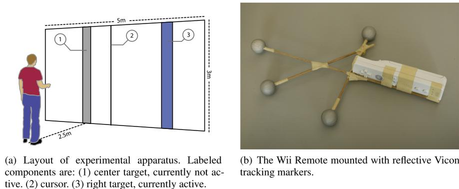
(a) Layout of experimental apparatus. Labeled components are: (1) center target, currently not active. (2) cursor. (3) right target, currently active.
