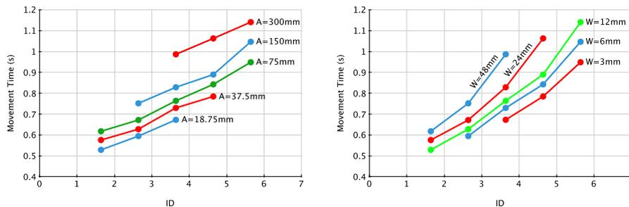
(a) Lines connect points representing tasks with the same movement amplitude  $A$ . (b) Lines connect points representing tasks with the same target width  $W$ .
