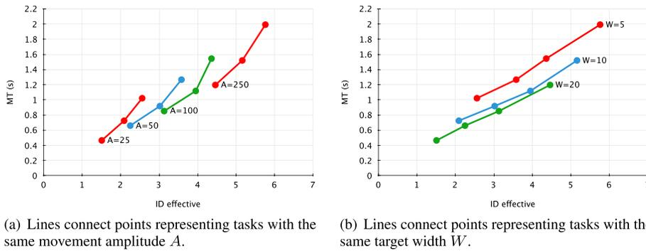
Fig. 9. Movement time results for all  $A$  and  $W$  combinations from the experimental data at  $G = 20$ . Data points in both graphs are the same. Effective target width was used in computing  $ID$ . An independent contribution of  $A$  and  $W$  to movement time is apparent, suggesting the need for a two-part linear model.
